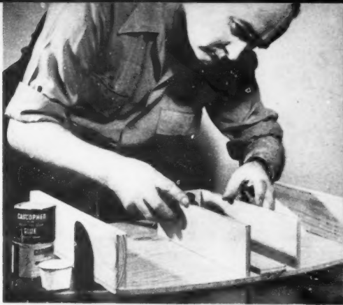
Gluing the light enclosure and side rails to the bottom of printer. Use clamps while glue sets.
